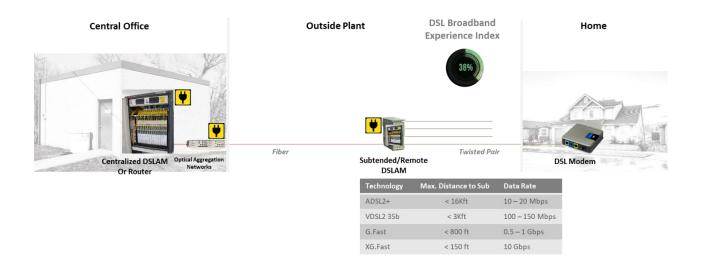
Figure 3 - DSL based access network architecture
