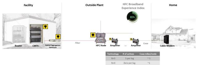
Figure 2 - Hybrid Fiber Coax-based access network architecture
