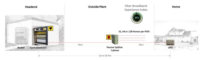
Figure 4 FTTH access network architecture
