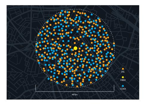
Figure 5 Typical powered equipment locations in a 40 Km area. Note the hundreds of powered nodes required for Coax and Copper based networks versus one powered location for FTTH. Each powered node is a potential network failure point
