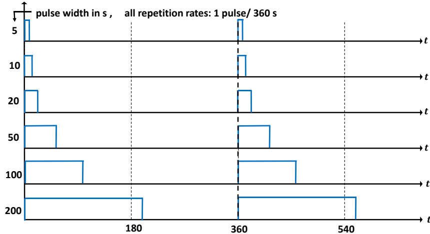
Fig. 5.24 , Examples of the first two periods of some of the continuous pulse trains used for testing the ICNIRP (2020) AED and APD OBRs.
