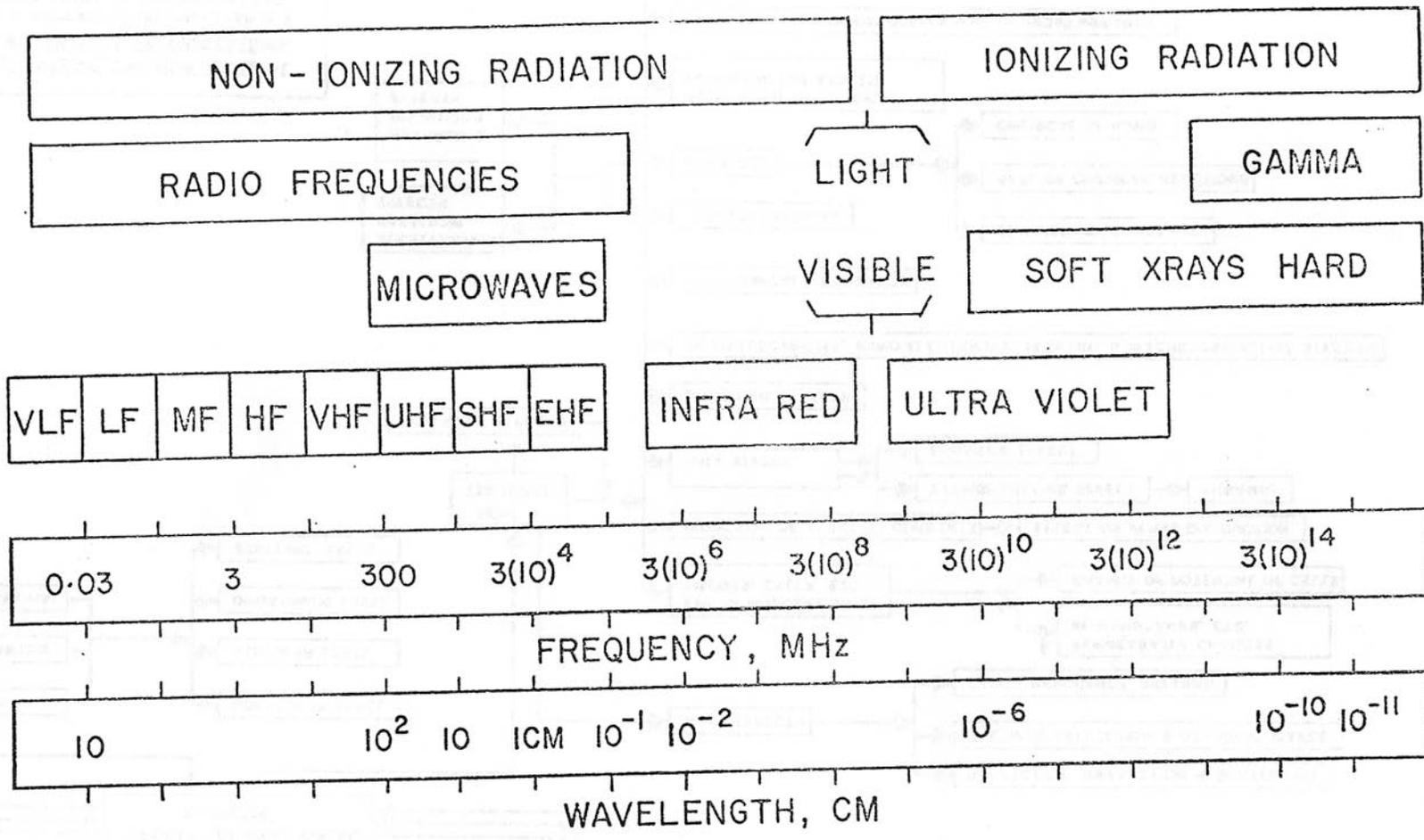
FIG.1: ELECTROMAGNETIC FREQUENCY SPECTRUM
