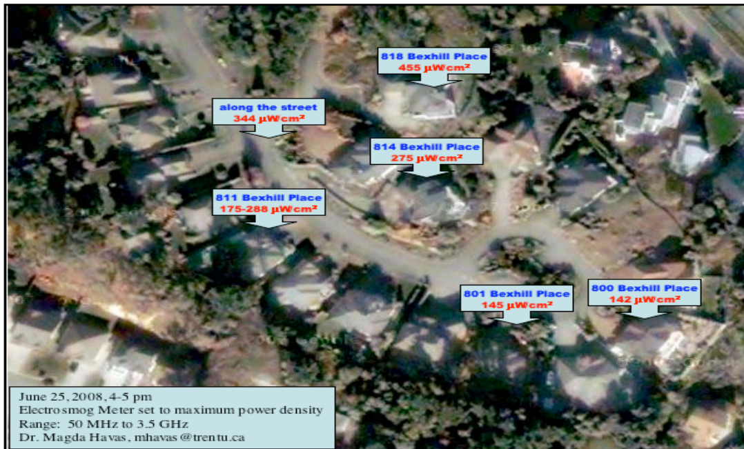
Figure 1. Satellite photograph of Triangle Mt with maximum power density readings at various homes taken on June 25, 2008 (google map).
