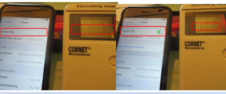
When LTE antenna is off, RF radiation at 0.0159 mW/m2 = 0.00159uW/cm2 When LTE is ON, RF radiation at 10,000X+ higher at 162.9 mw/m2 = 16.29uW/cm2
