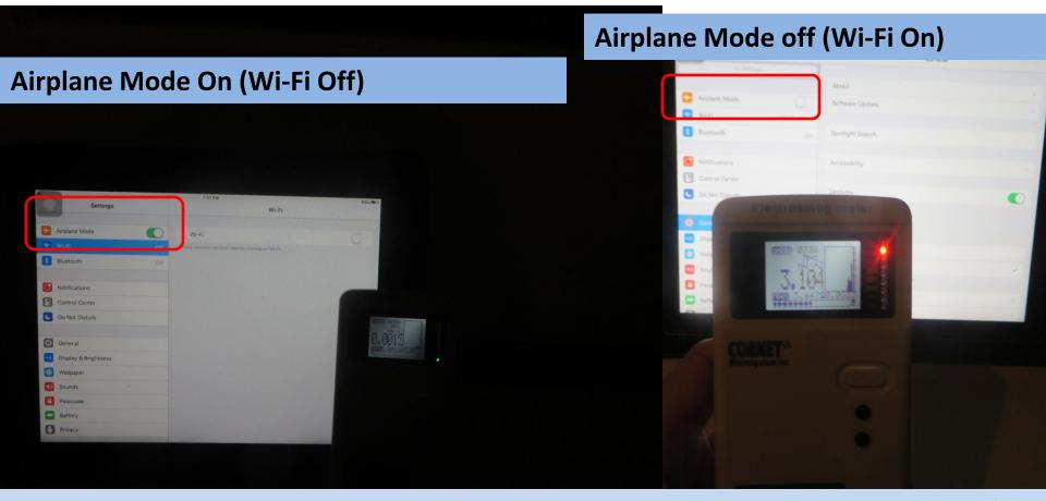
When Airplane Mode On (Wi-fi off), RF radiation is at ambient levels, 0.0015 mW/m2. When Airplane Mode Off (Wi-fi on), RF over 2000X higher at 3.104 mW/m2 = 0.3104uW/cm2.
