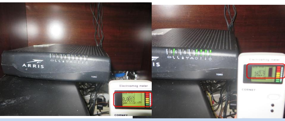
When wi-fi is off, RF radiation is at ambient levels for the room, 0.0010 mW/m2. When wi-fi is on, RF over 10,000X higher at 162.9 mW/m2 = 16.29 uW/cm2.
