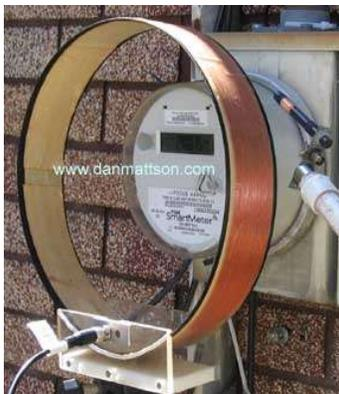
These are the two antennas I used for the measurement of the radiated emissions from the SMPS. I made the loop antenna about five years ago. It is about 12 inches in diameter and has about 120 feet of 18-gauge wire wrapped in a single layer. I had the opportunity to compare it to a high-end loop antenna. It compared well. I have no calibration data on it, but it works best as a 50-ohm antenna. It is usable from ELF to about one GHz. It is best from about 1MHz to 30 MHz.
