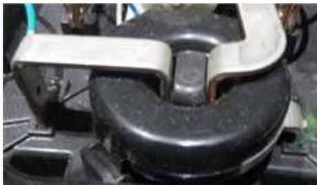
An electricity meter, either analog or digital, produces an ELF magnetic field proportional to the current being drawn through the meter by end user loads. In the case of an analog meter the motor that spins the familiar disc produces this field. In the digital meter, such as this smart meter, a current transformer produces the field. This is the same technology as the clamp-on current clamps used in Part Two.
