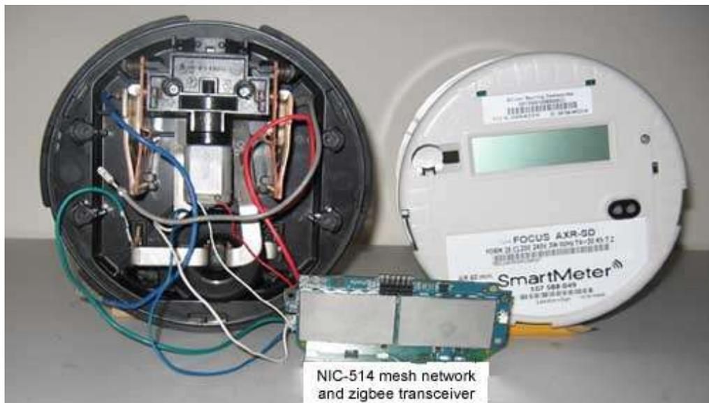
**A safe smart meter.** This was left, partially disassembled, in a box on my doorstep. It has been valuable and interesting to get an inside view of this thing that is making so many people sick, but I have not gone so far as to connect power to it.
