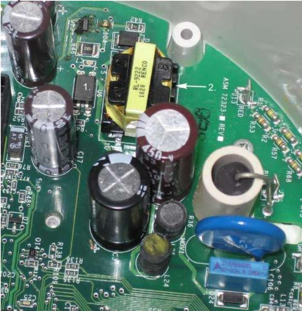
This shows the section of the circuit board that holds the power supply and surge protection components. The SMPS seems to be a fairly ordinary 12-volt DC one-amp power supply. The current waveform shown on page five indicates little was done to address power factor (discussed on p. 4).
